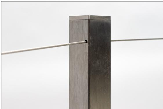
Guide the tensioning ropes through the middle posts at the top and the bottom. At one side insert the ropes into the rope tensioner
