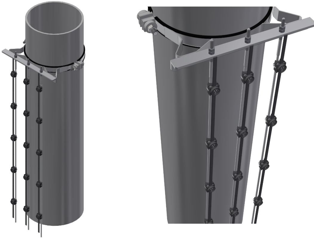
LED-Dot on stainless clip with stainless steel bracket fixed on twin ropes Ø 2,0mm and pipe clamp
